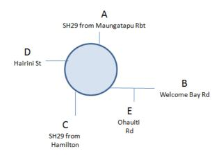
**Pre-Signal Performance:** Regular and severe congestion occurred on the Welcome Bay approach (Arm B) in the AM peak period and on the northern SH29 approach (Arm A) in the PM peak period. The latter regularly led to block-back to the Maungatapu roundabout, causing serious congestion in the PM peak there also.
