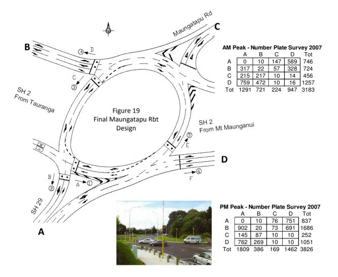
**Signal Control in Operation:** This is illustrated below for the AM peak period. A particular feature to note is that there is about 22" (AM Peak) and 10" (PM Peak) of wasted green time purposely introduced at the Arm B (SH2 from Tauranga city) gyratory stopline (*i.e. the last car from the SH29 Welcome Bay approach will pass the SH2 (City) stopline at about 7". The SH2 (City) approach does not receive green until 29", some 22" later).* This 'wasted green time' serves two purposes:-
