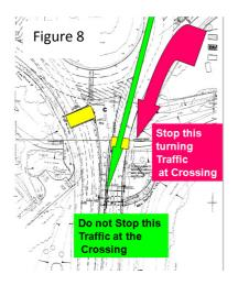
It is generally safest to 'hard-link' exit crossings to the roundabout, i.e. include them in the linking plan. The linked timing must endeavor to achieve:-
