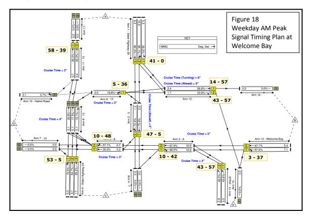
WB Signal Control in Operation: The LinSig CLF Plan for the AM peak period at WB is as follows:-
